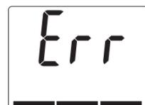
**Scale will show "Err" if there is improper foot contact in the body analysis mode, for instance, when you stand on the scale with socks or shoes on. Hard or dry skin can prevent you from making proper contact with electrodes on the surface of the scale. Try applying a small amount of moisturizer to your feet before using the scale.**
